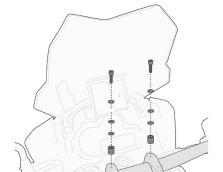
01SKITK Specific kit to mounting the KS900A Smart Bar
