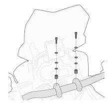
02SKITK Specific kit to mounting the KS900A Smart Bar
