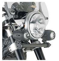
LS9058K Specific fitting kit to mount spotlights where specific engine guard is not present
