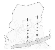
05SKITK Specific kit to mounting the KS900A Smart Bar
