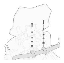
015KITK Specific kit to mounting the KS900A Smart Bar
